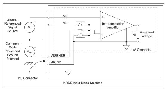
Figure 2-8. Single-Ended Input Connections for Ground-Referenced Signals
